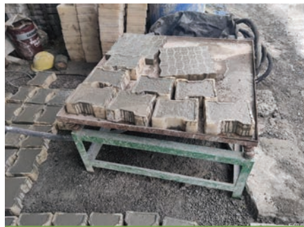
Paver blocks from recycled concrete waste
